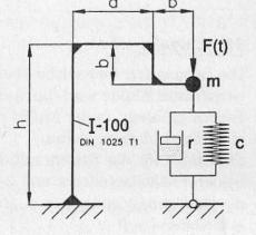
$\frac{\text{Geg.:}}{c = 5,5 \cdot 10^5 \text{ N/m}, \ F_0 = 1250 \text{ N}, \ \alpha = 5, \Omega = 50 \cdot \pi, \ E = 2,1 \cdot 10^{11} \text{ N/m}^2.}$
